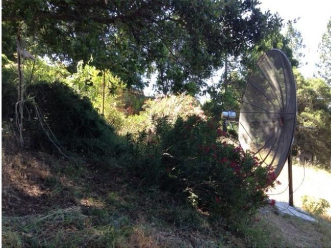
Data was obtained over a 48 hour period during which the measured power range was from - 26.66 dB ( $pwr = 2.16 * 10^{-3}$  pu) to -26.34 dB. The measured temperature range of the shrubbery toward which the antenna was pointed was  $T_{WE} = 296$  K to 304 K. The  $T_{WE}$  average was 300 K and average power was  $2.29 * 10^{-3}$  pu where the pu is an arbitrary unit of power.
